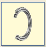
Crossed Roller Bearings are high-rigidity and compact bearings with their cylindrical rollers alternately crossed at right angles to each other between inner and outer rings. A single Crossed Roller Bearing can take loads from any directions at the same time such as radial, thrust, and moment loads.
