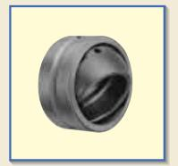
Spherical Bushings are self-aligning spherical plain bushings, which have inner and outer rings with spherical sliding surfaces. They can take a large radial load and a bi-directional axial load at the same time.
