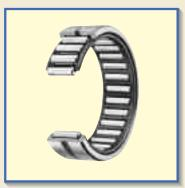
Machined Type Needle Roller Bearings have an outer ring made by machining, heat treatment, and grinding. The outer ring has stable high rigidity and can be easily used even for light alloy housings.
