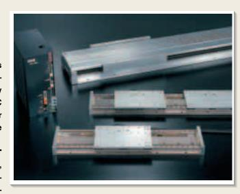
vides a high thrust of 450N though its height is only 40 mm. The moving table is as light as 1.5 kg but provides high thrust. It permits high acceleration and deceleration exceeding 10 G. (In the case of LT150 CG.) Also, High Thrust Series LT... H outputs 900N thrust.
