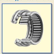
Combined Type Needle Roller Bearings are combinations of a radial bearing and a thrust bearing. Caged Needle Roller Bearings are used as radial bearings and Thrust Ball Bearings or Thrust Roller Bearings are used as thrust bearings.
