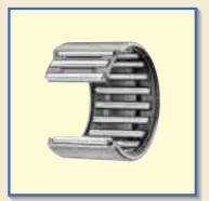
Shell Type Needle Roller Bearings are lightweight with the lowest sectional height among needle roller bearings with outer ring, because they employ a shell type outer ring made from a thin special-steel plate which is accurately drawn, carburized and quenched.
